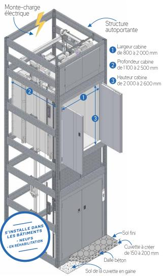
i Conforme aux normes EN81-31 / directive machine 2006/42/CE
